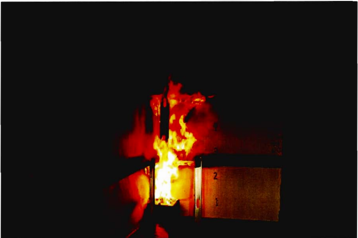
Figure B-4. Burner Increased to 160 kW.
